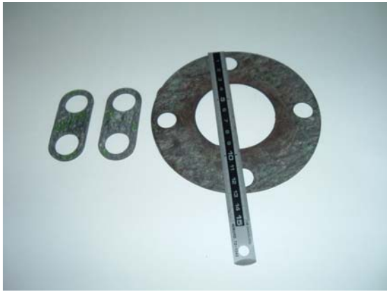
Fig. 10. Asbestic gaskets for joint sealing
