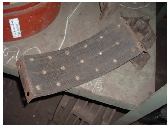
Fig. 9. Asbestos brake-lining in crane
