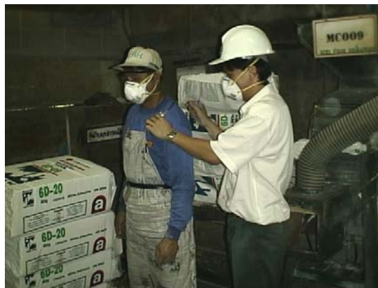
Figure 1. Personal air sampling for asbestos
